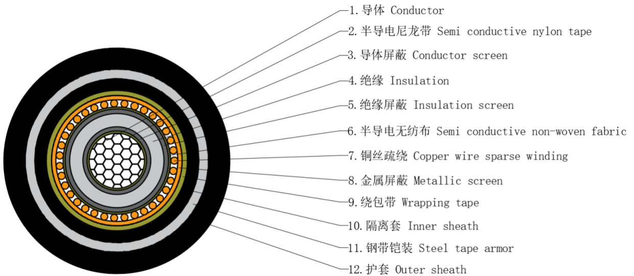
单芯钢带铠装电力电缆 1-core conductor steel tape armor power cable
